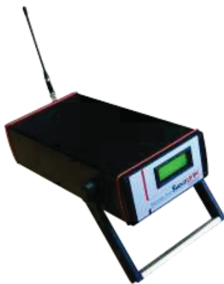
ShortLINK-Receiver with "in-" or "out-door" antenna
